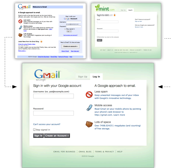
Figure 1. Bricolage computes coherent mappings between Web pages by matching visually and semantically similar page elements. The produced mapping can then be used to guide the transfer of content from one page into the design and layout of the other.
