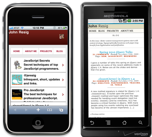
Figure 11. Bricolage can retarget Web pages designed for the desktop to mobile devices. Left: the original Web page. Right: the page automatically retargeted to two different mobile layouts.
